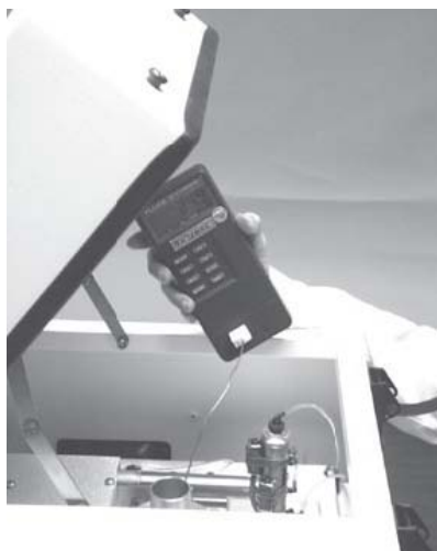
Figure 11: 2025i – Inserting an External Temperature Probe into the Sampling Chamber
